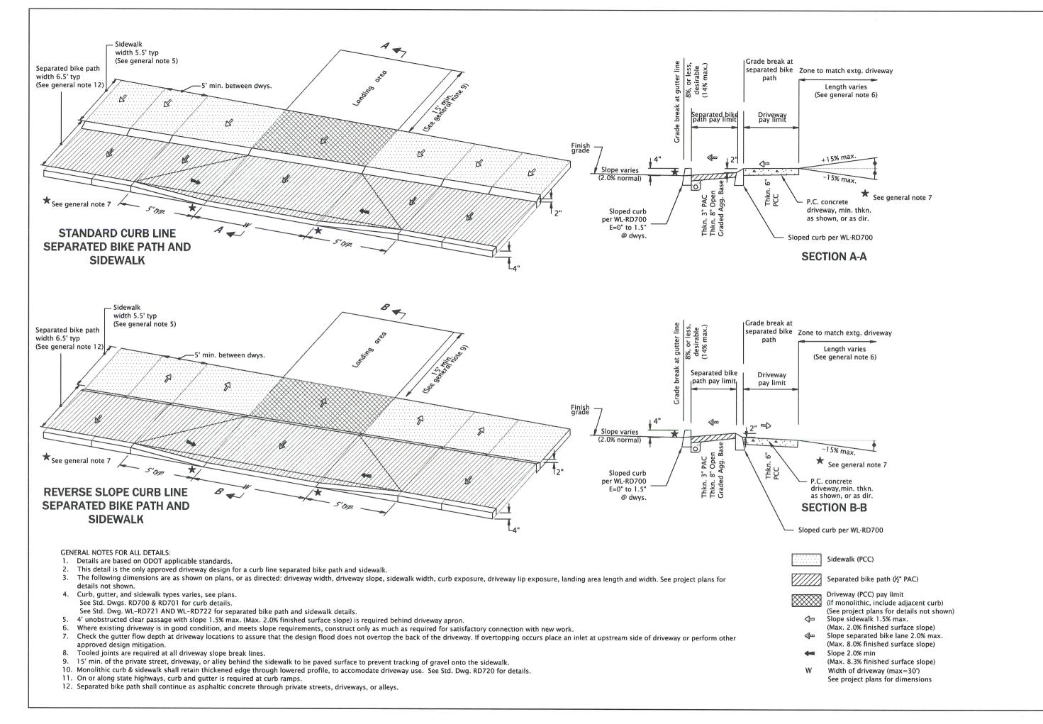
ROADS, OR ALLEYS AT CURB LINE SEPARATED BIKE PATH AND SIDEWALK
