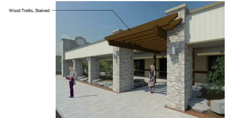
④ VIEW OF TRELLIS N.T.S. Signage Not Shown
