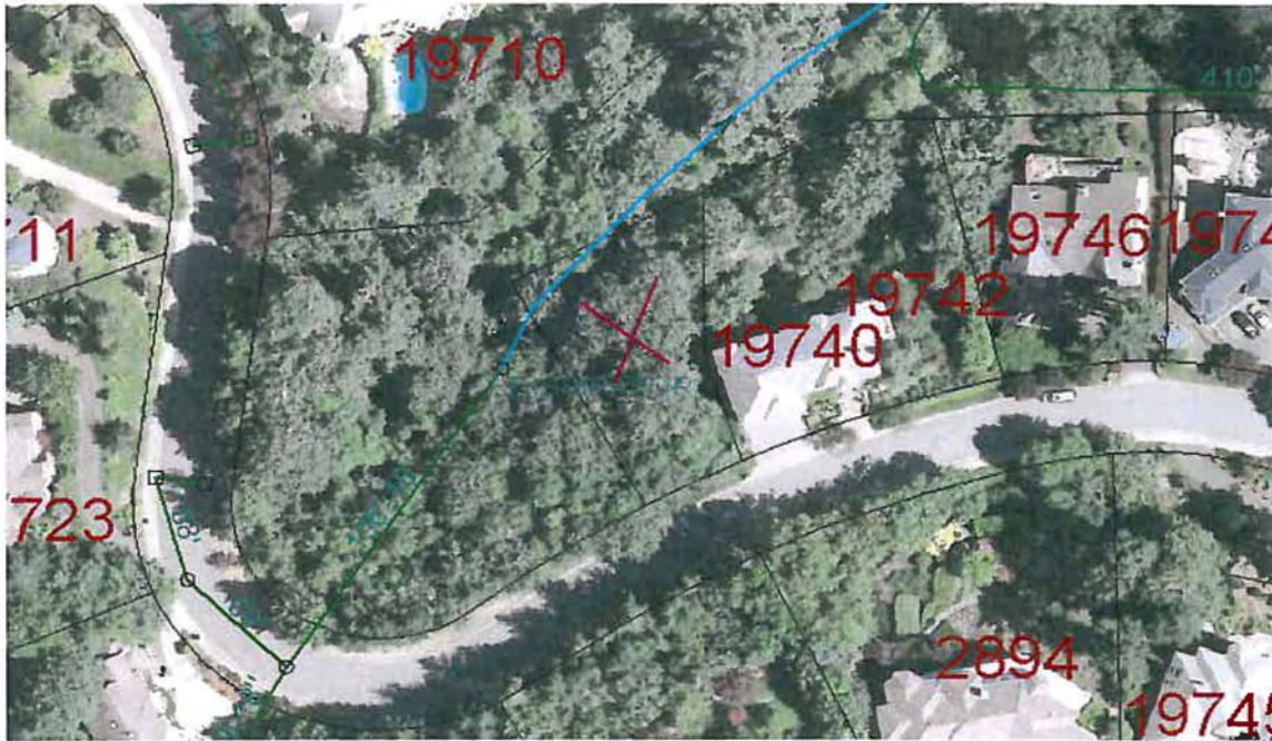
Site/Vicinity Aerial Photo (Site with purple “x”, the drainageway in blue line, which drains from a stormwater pipe represented by the green line)
