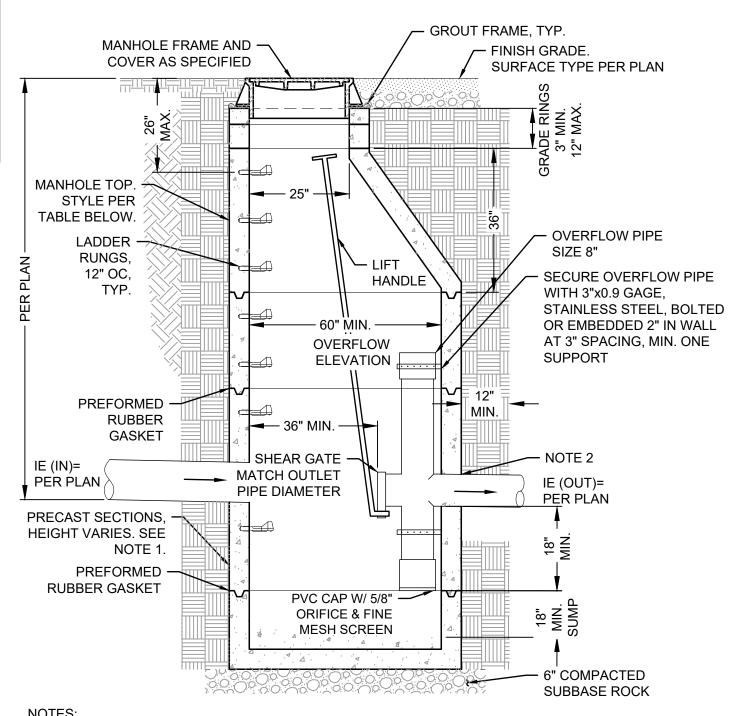
ALL PRECAST SECTIONS SHALL CONFORM TO REQUIREMENTS OF ASTM C-478.
