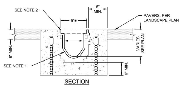
1. TRENCH DRAIN SHALL BE PRE-SLOPED 4" WIDE ZURN OR ACO TRENCH DRAIN OR APPROVED EQUAL.
