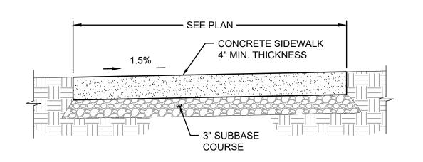
CONSTRUCT CONTRACTION JOINTS AT 15' MAX. SPACING AND AT RAMPS. CONSTRUCT EXPANSION JOINTS AT 200' MAX SPACING, AT POINTS OF TANGENCY AND AT ENDS OF EACH DRIVEWAY, UNLESS NOTED OTHERWISE.
