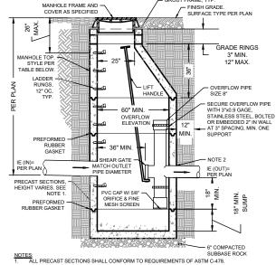
ALL CONNECTING PIPES SHALL HAVE FLEXIBLE, GASKETED AND UNRESTRAINED JOIN'
