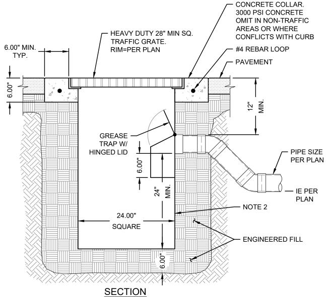
CONTRACTOR TO WIDEN EXCAVATION AS REQUIRED TO OBTAIN COMPACTION WITH CONTRACTORS COMPACTION EQUIPMENT.
