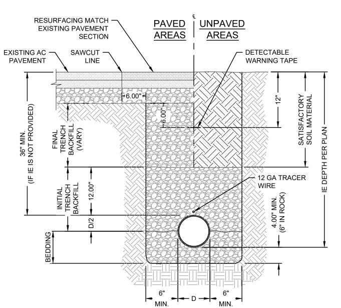
TYPICAL PIPE BEDDING AND BACKFILL
