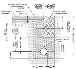
TYPICAL PIPE BEDDING AND BACKFILL
