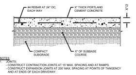
REINFORCED CONCRETE PAVEMENT SECTION
