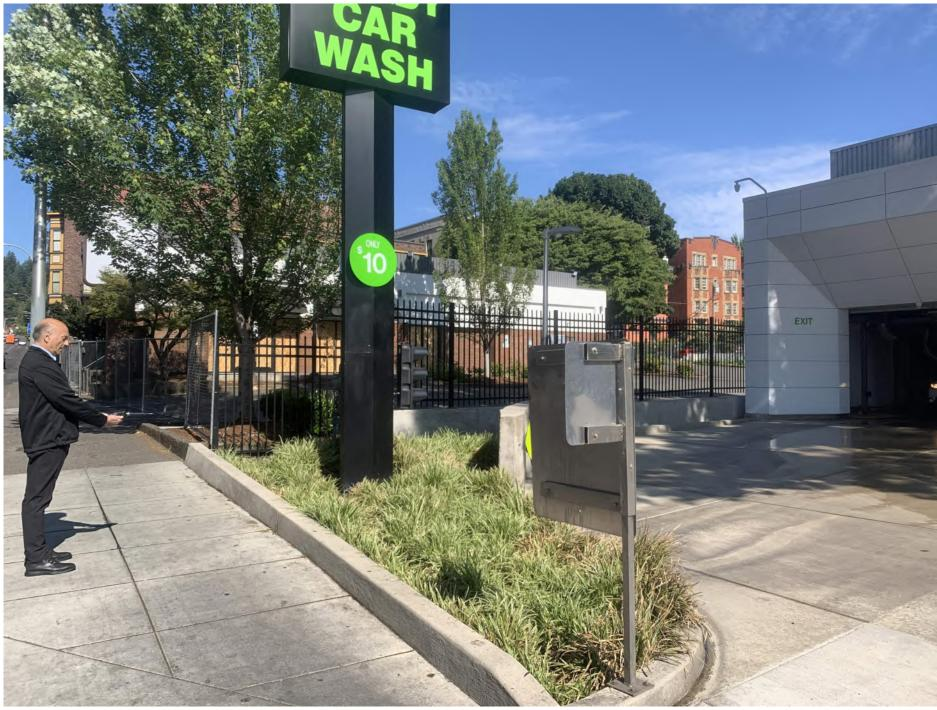
Decibel readings taken at 50'-0" from the car wash exit: 72 db to 80 db (Including background noise from Burnside) SHOWN Decibel readings taken at 42 feet from the car wash entry on the north side: 72 db
