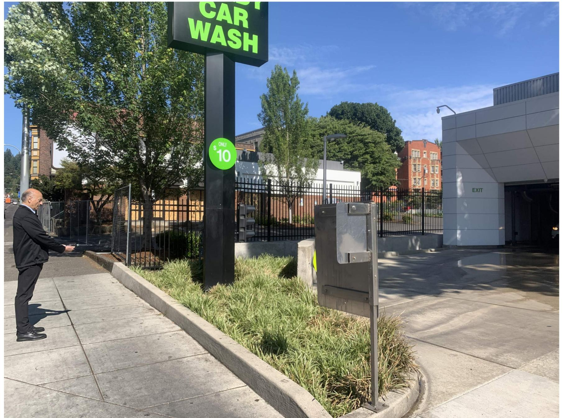
Decibel readings taken at 50'-0" from the car wash exit: 72 db to 80 db (Including background noise from Burnside) SHOWN
