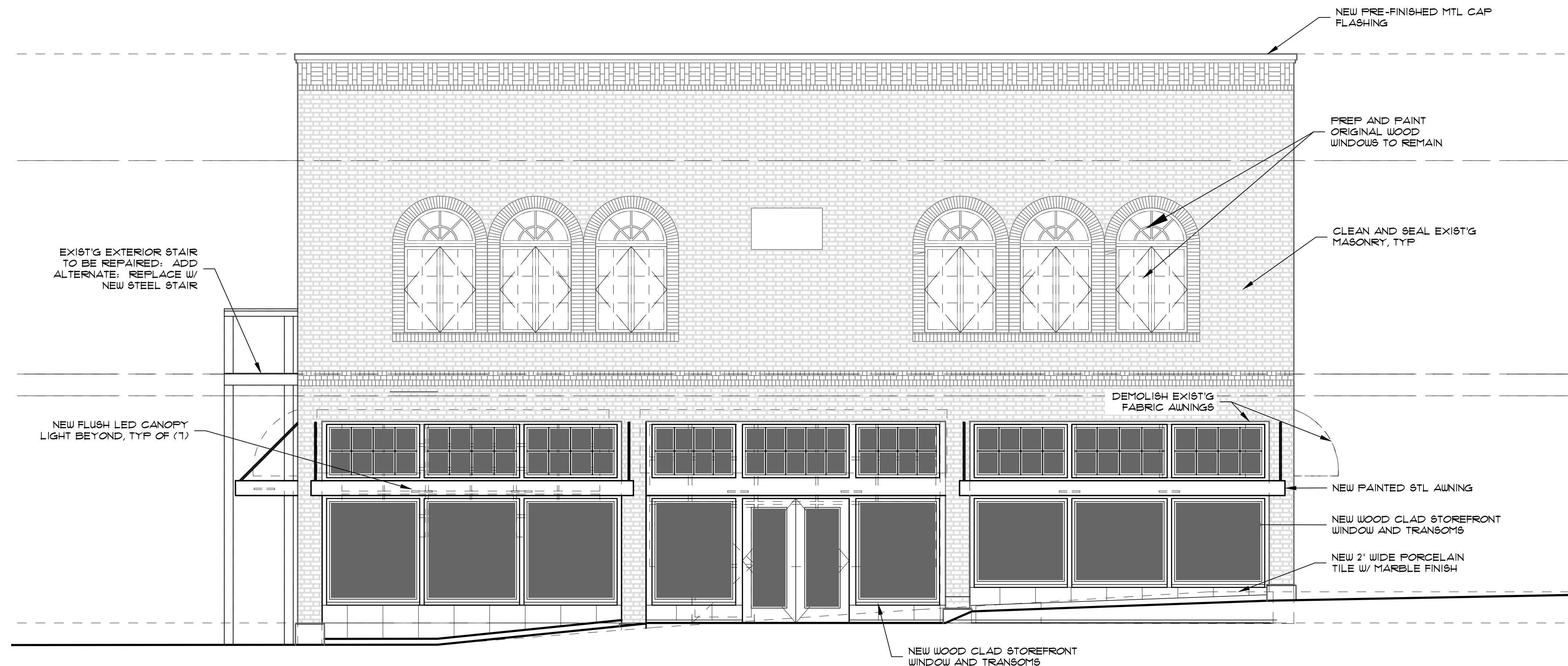
NORTHEAST (FRONT) ELEVATION
