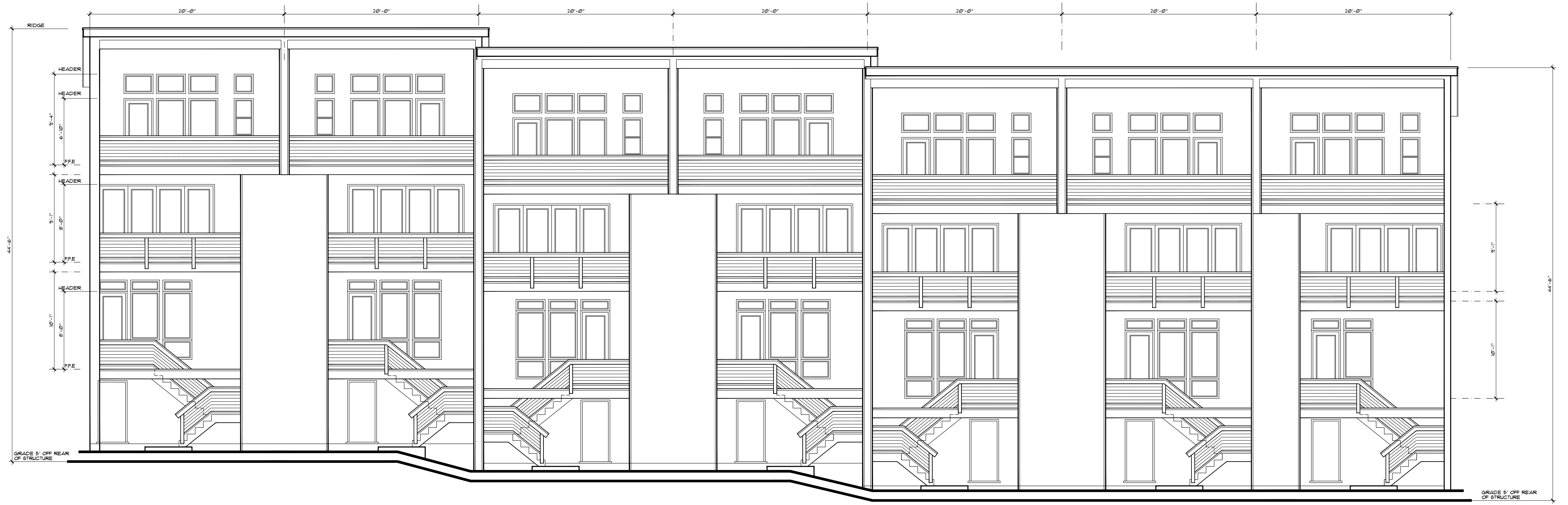
REAR ELEVATION - EAST SCALE: 1/4" = 1'-0"
