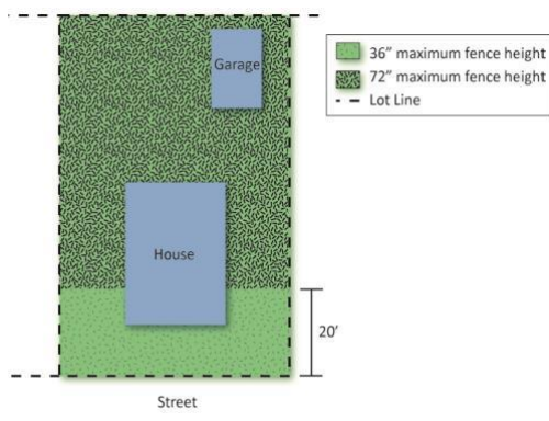
Figure 1: Example of Exempt Interior Lot Fence Locations
