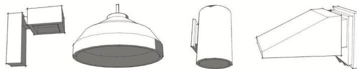
Examples of shielded light fixtures
