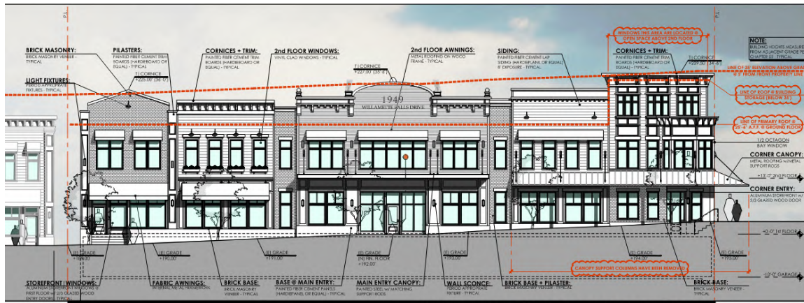
WILLAMETTE FALLS DRIVE ELEVATION
