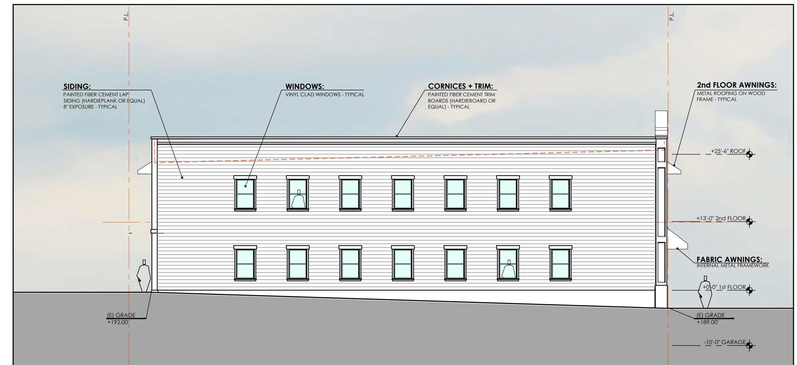
EAST (INTERIOR P.L.) ELEVATION
