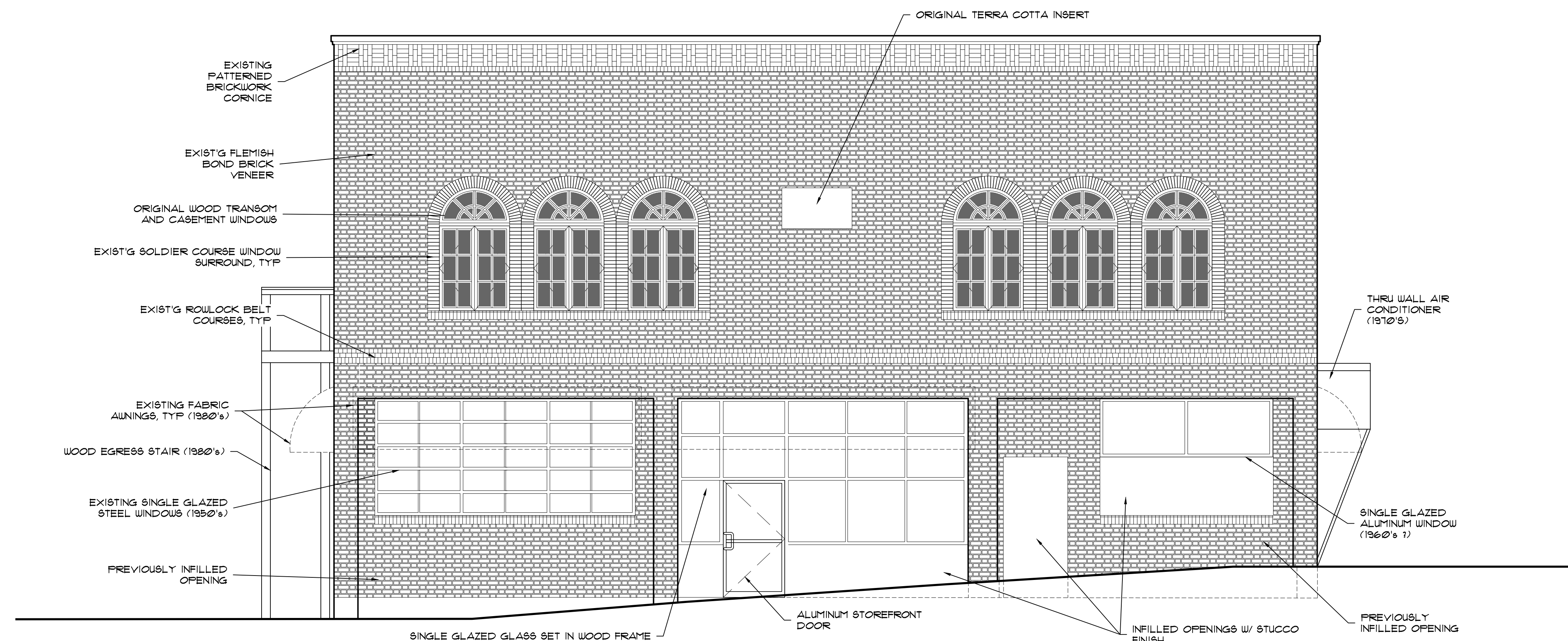
NORTHEAST (FRONT) ELEVATION
