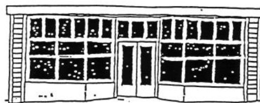
MULTI-PANED PEDESTRIAN LEVEL WINDOWS
