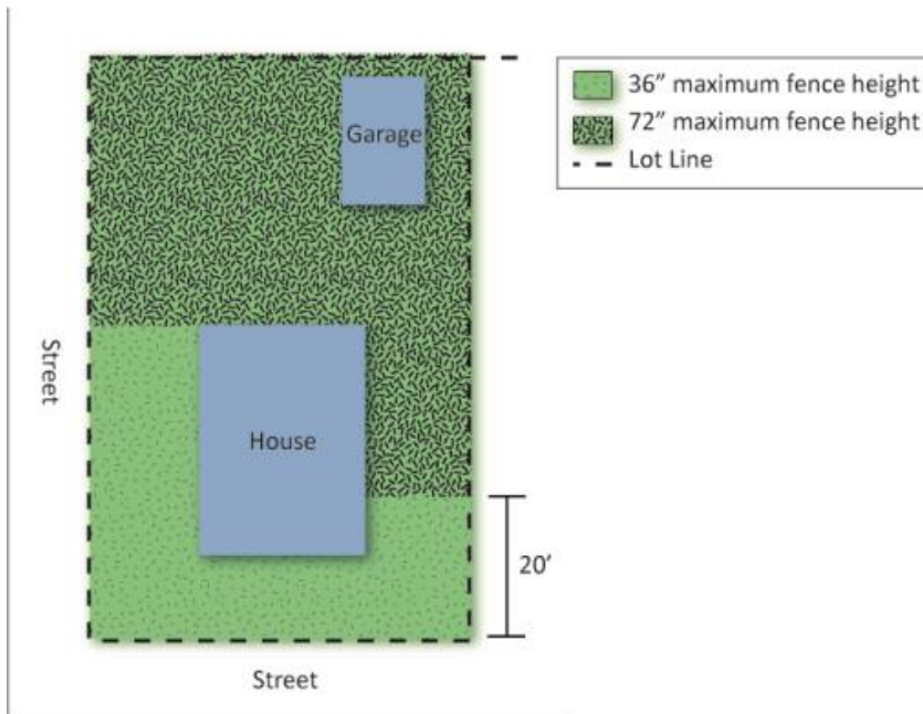
Figure 2: Example of Exempt Corner Lot Fence Locations
