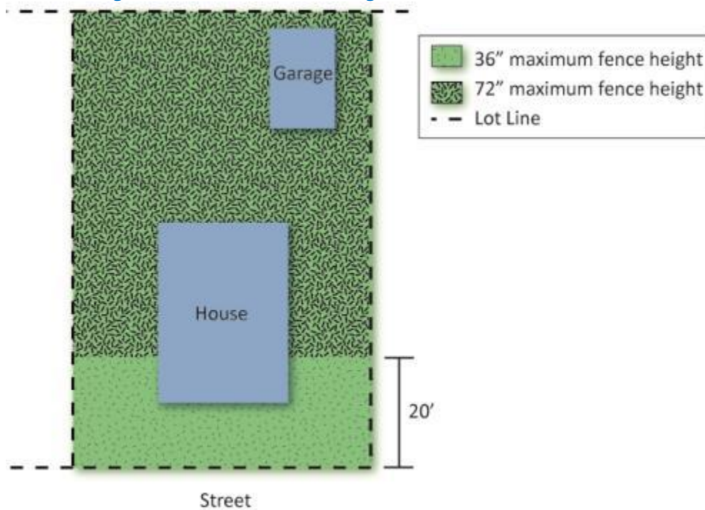
Figure 1: Example of Exempt Interior Lot Fence Locations
