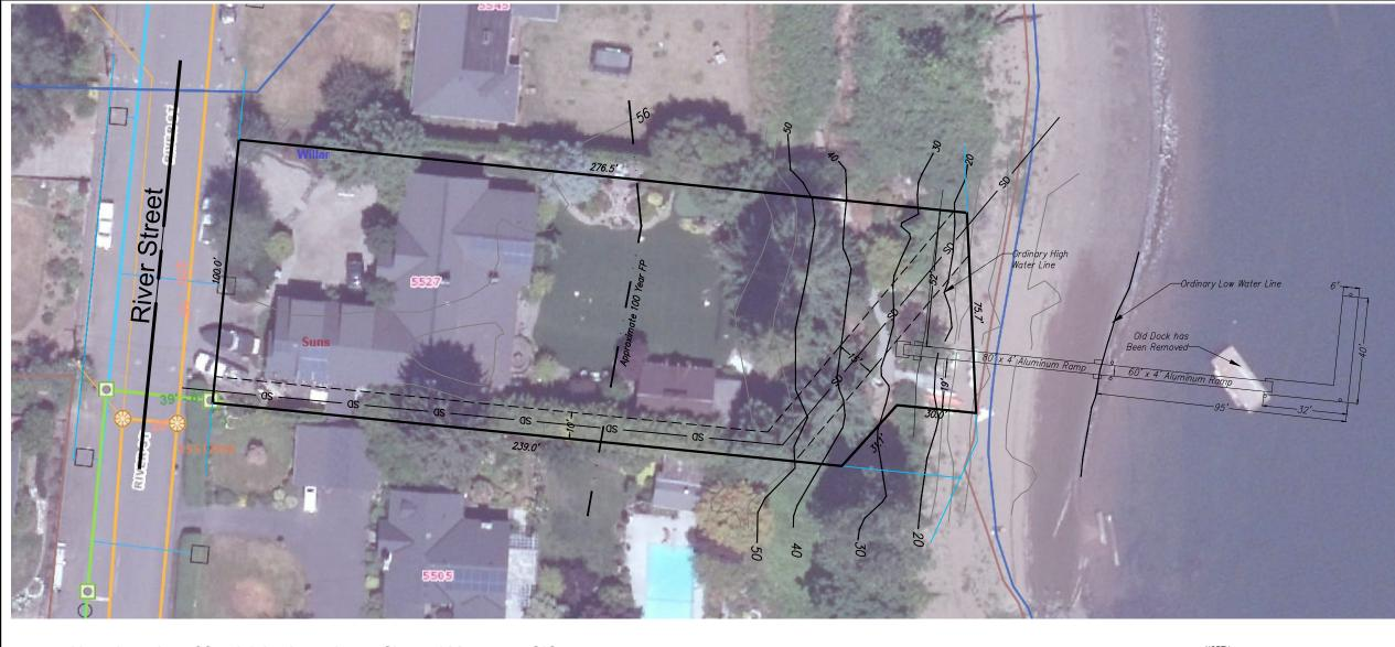
Note: Location of floodplain shown is per City and Metromap GIS. Base flood elevation per FEMA Flood Panel 41005C0276D is approximately 48.2' NAVD 88.
