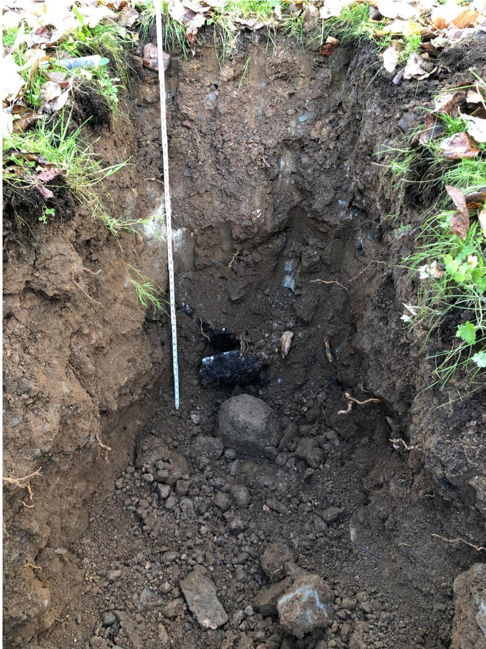
Test Pit TP-1 Undocumented Fill
