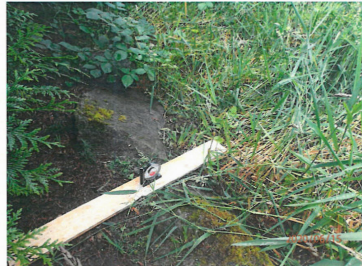
Measuring slope from WRA boundary to landscaped area and residence on site which was noted on average of less than 5% slope.
