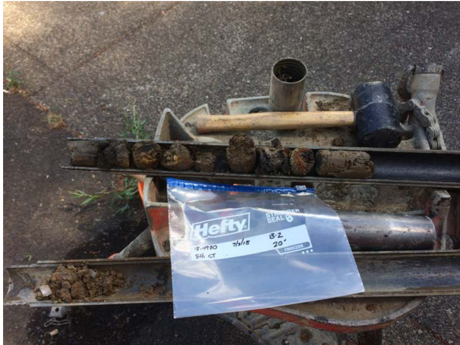
Boring B-2, Bedrock Encountered at 20.9 Feet bgs
