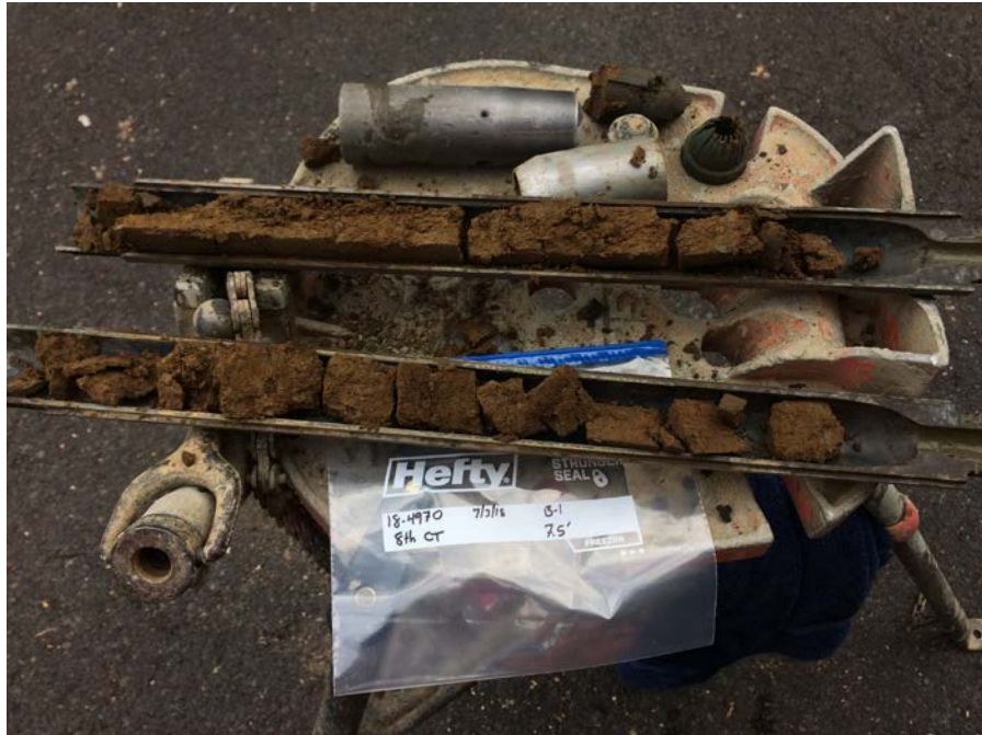
Boring B-1, Contact to Native Soil at 6.3 feet bgs.
