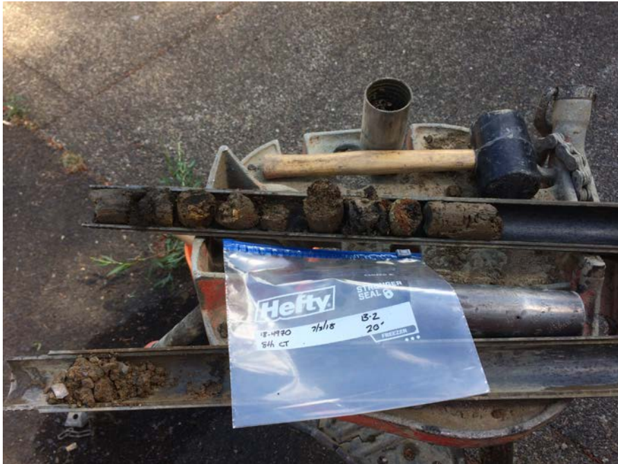
Boring B-2, Bedrock Encountered at 20.9 Feet bgs
