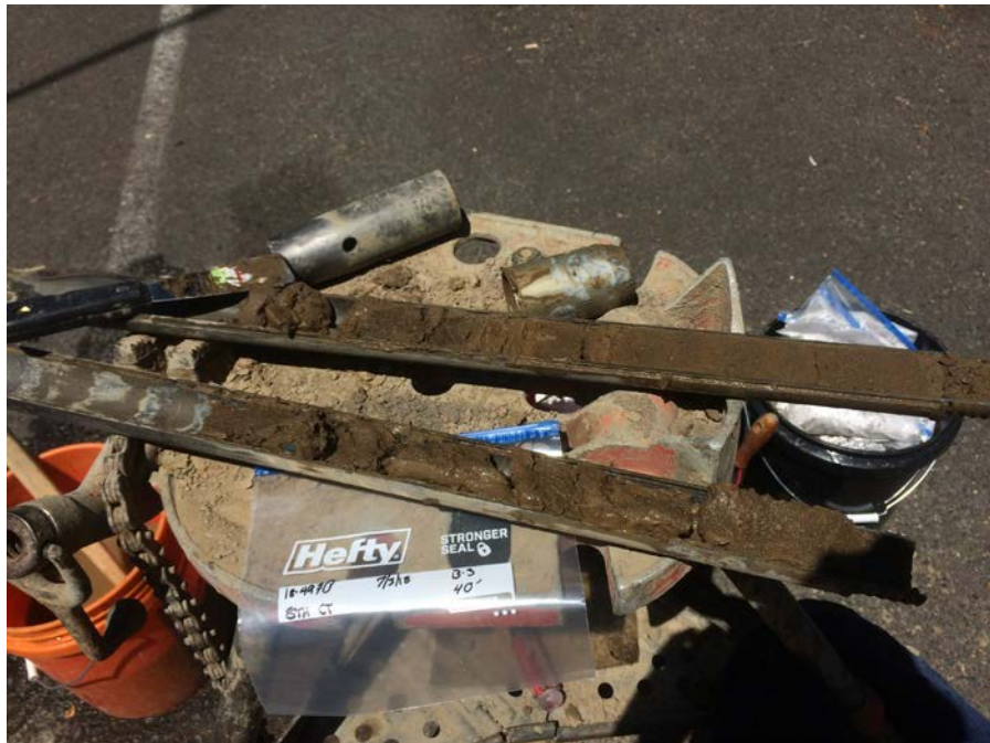
Boring B-3, Potentially Liquefiable Soil at 40 Feet bgs
