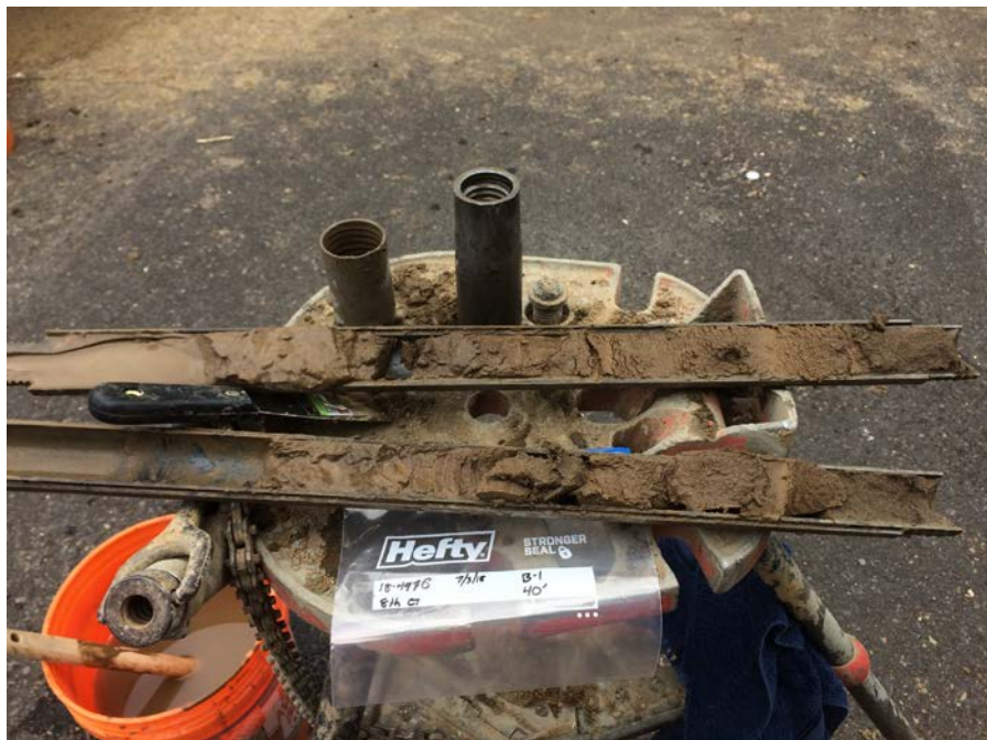
Boring B-1, Potentially Liquefiable Soil at 40 Feet bgs
