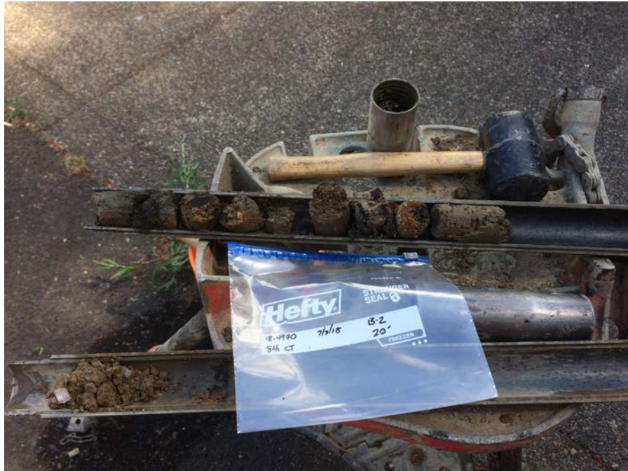
Boring B-2, Bedrock Encountered at 20.9 Feet bgs
