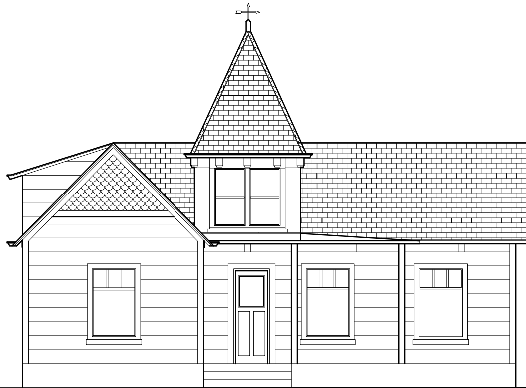
1 EXISTING EXTERIOR SOUTH ELEVATION SCALE: 1/8" = 1'-0"
