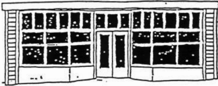
MULTI-PANED PEDESTRIAN LEVEL WINDOWS
