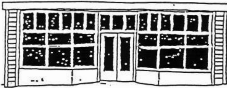
MULTI-PANED PEDESTRIAN LEVEL WINDOWS
