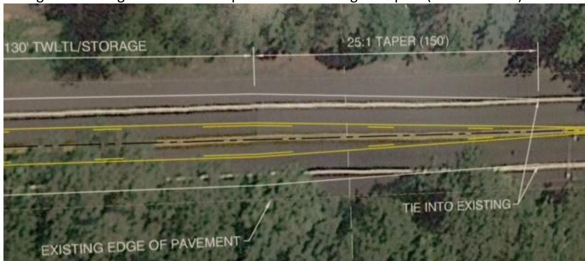
Enlargement of Figure 9 above: Proposed interim mitigation plan (southern end)
