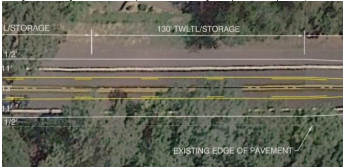
Enlargement of Figure 9 above: Proposed interim mitigation plan (southern end)
