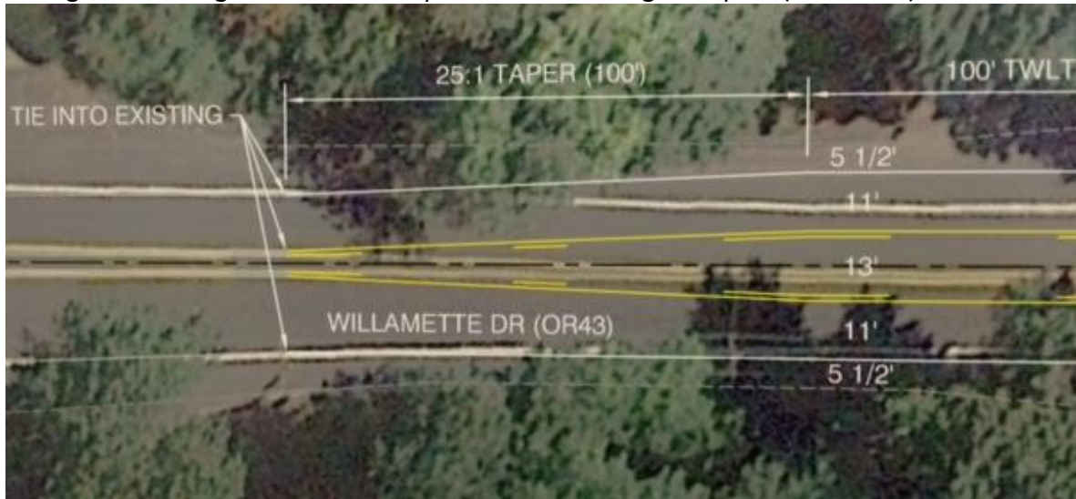
Enlargement of Figure 9 above: Proposed interim mitigation plan (Arbor Drive intersection)
