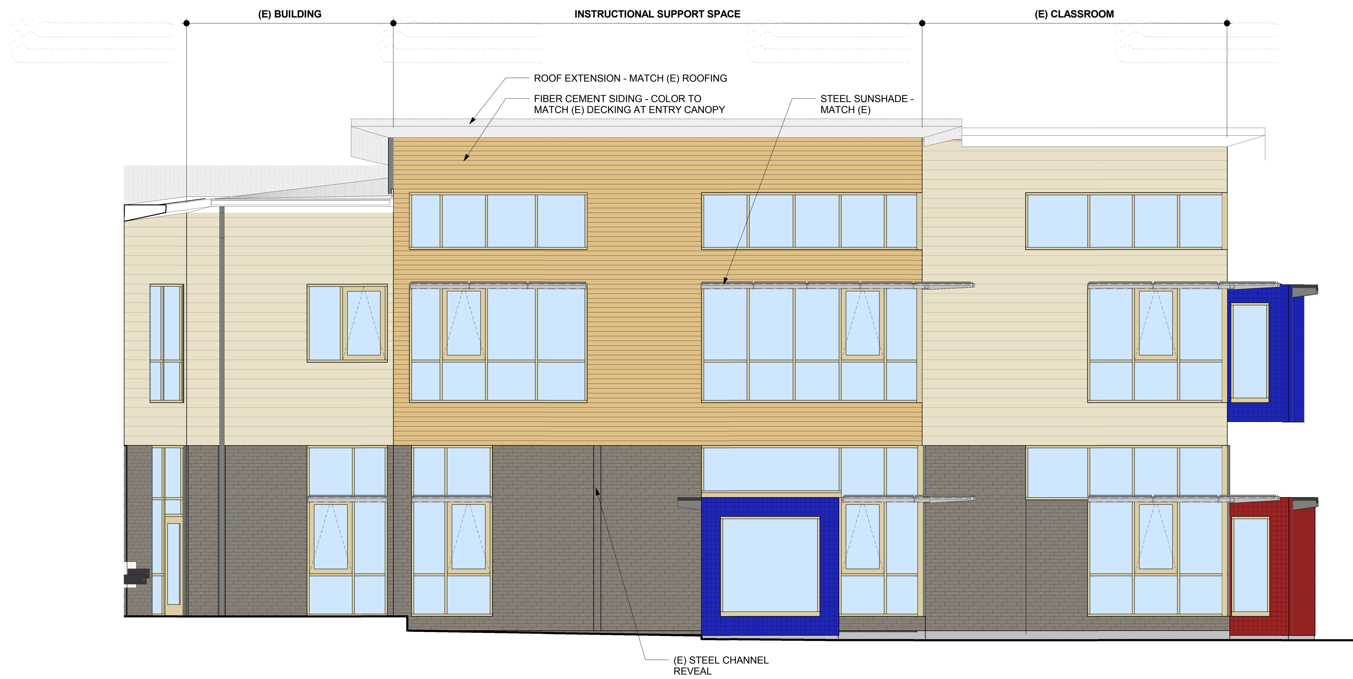
EXTENDED LEARNING ADDITION - EAST ELEVATION ④ SCALE: 1/4" = 1'-0"
