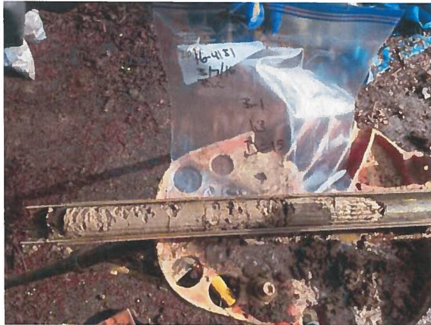
Split Spoon Sample, Soil Boring B-1, Depth = 15 Feet
