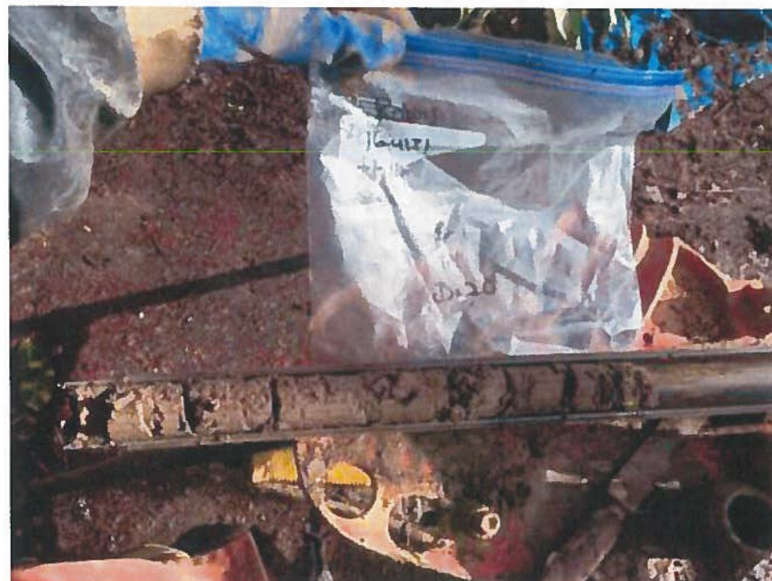
Split Spoon Sample, Soil Boring B-1, Depth = 20 Feet
