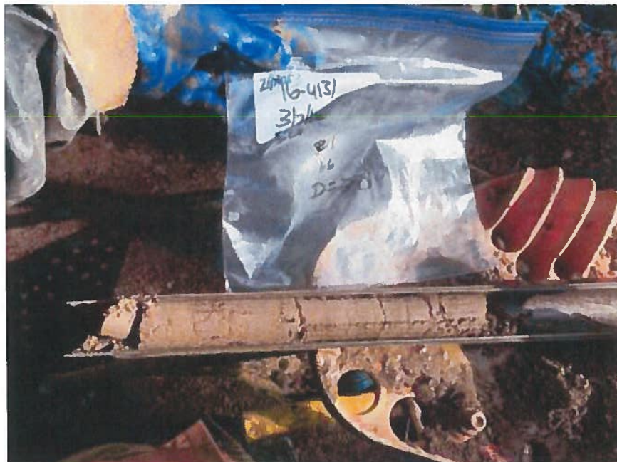
Split Spoon Sample, Soil Boring B-1, Depth = 30 Feet
