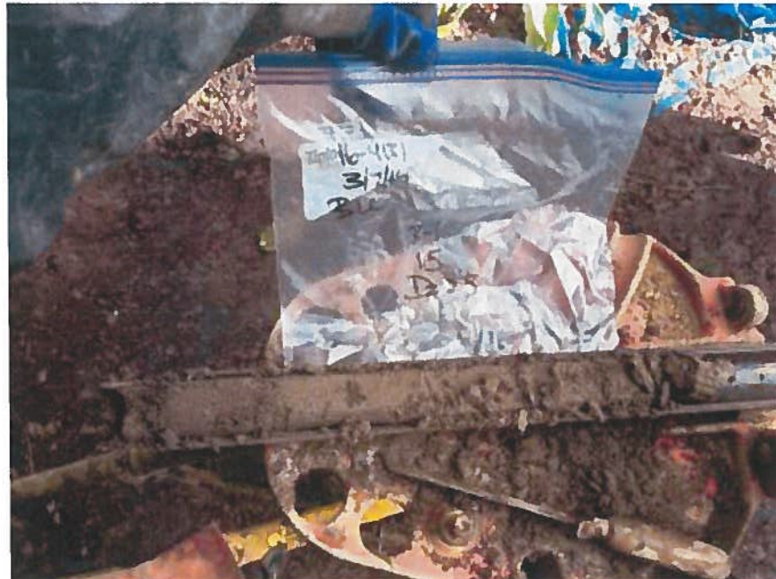
Split Spoon Sample, Soil Boring B-1, Depth = 25 Feet
