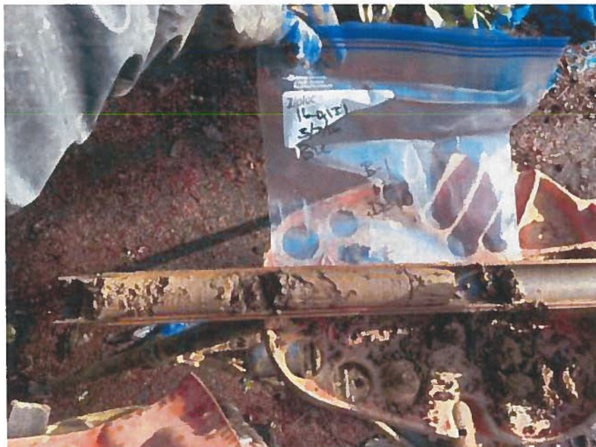
Split Spoon Sample, Soil Boring B-1, Depth = 10 Feet
