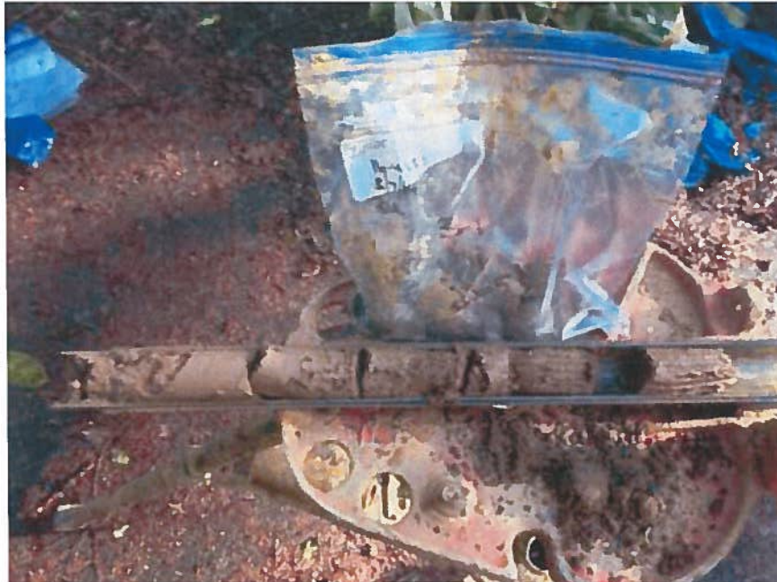
Split Spoon Sample, Soil Boring B-1, Depth = 5 Feet
