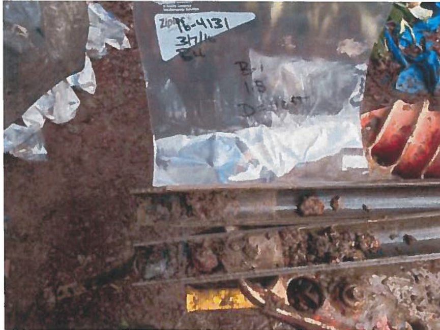
Split Spoon Sample, Soil Boring B-1, Depth = 40 Feet
