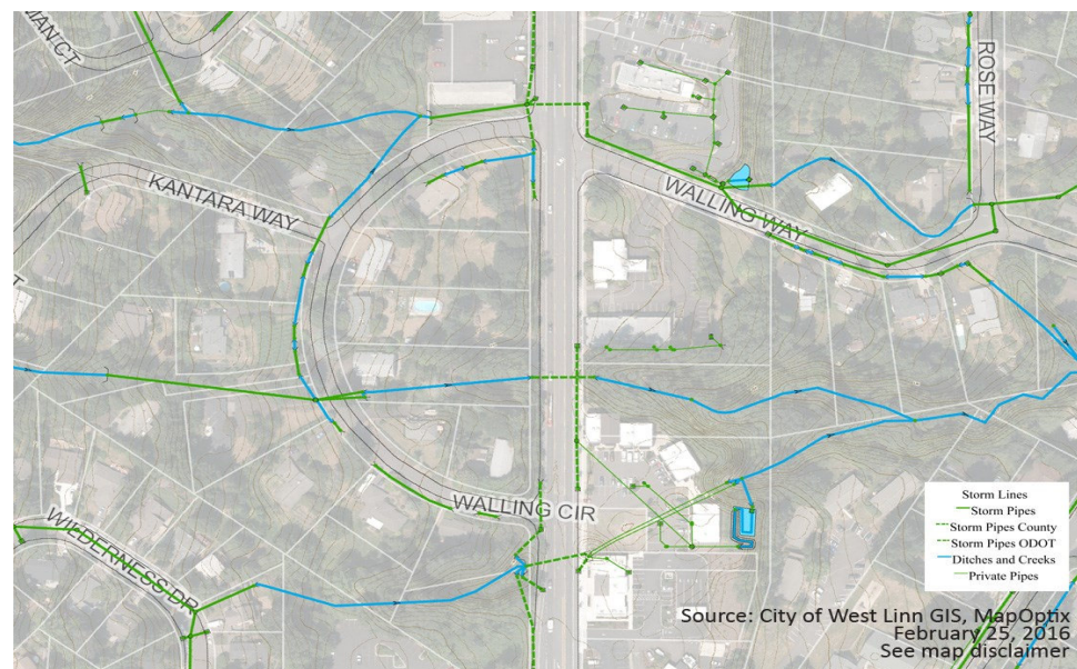
Example of some of the existing Stormwater facilities and drainage impacting the OR 43 corridor
