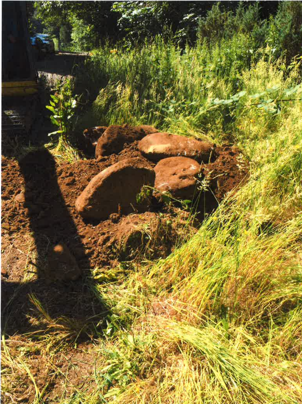
Fill Material Consisting of Boulders in Test Pit TP-4
