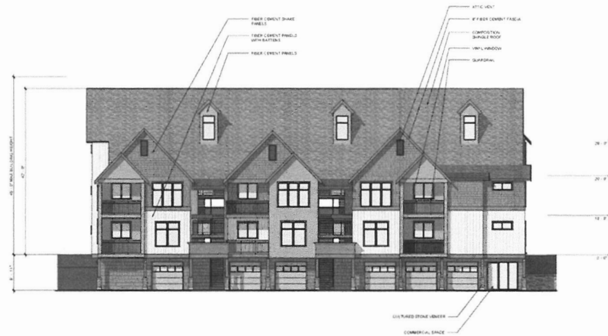
BUILDING TYPE 5 BACK ELEVATION SCALE: 1/8" = 1'-0"
