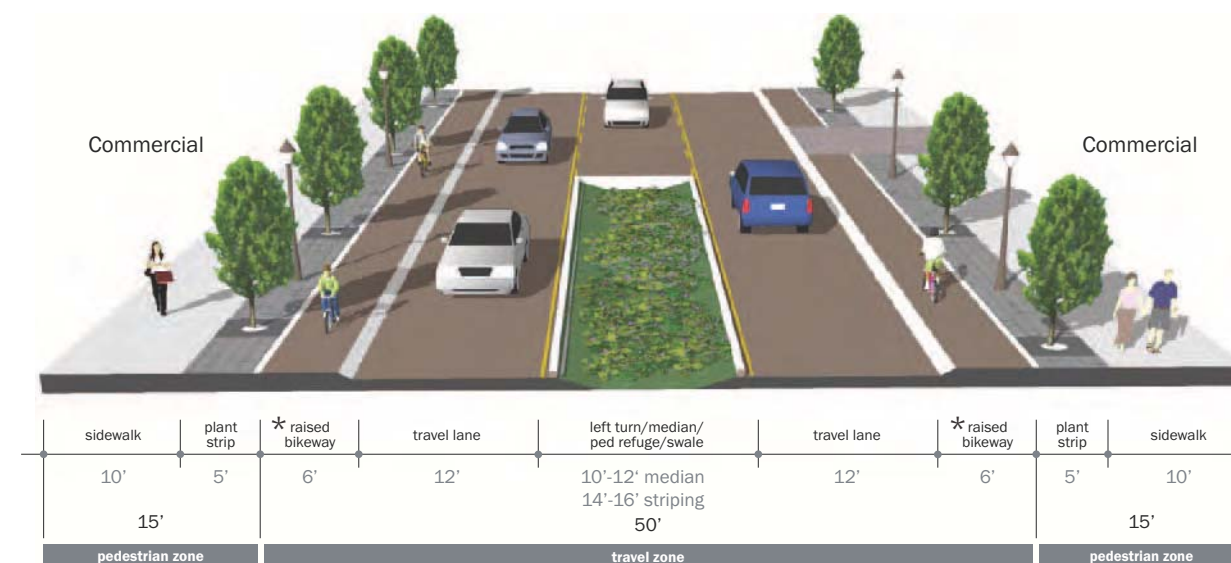
Example of proposed raised bike facility
