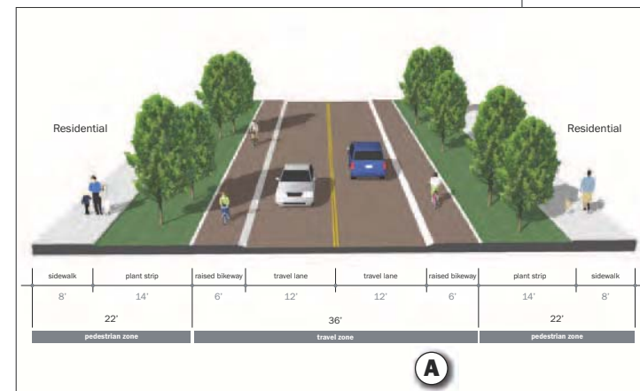
A typical cross-section designed for residential areas
