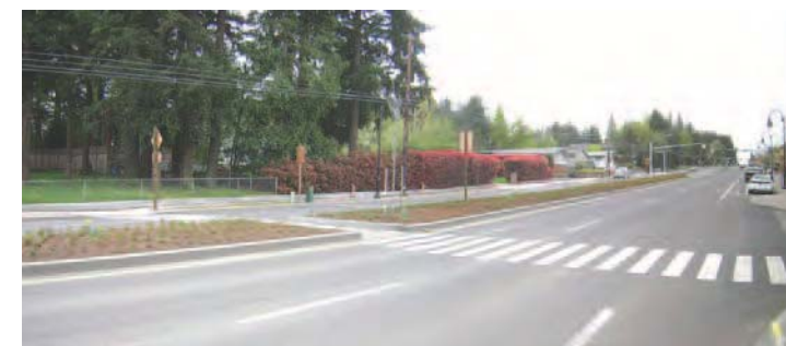
Pedestrian refuge and median crossing examples
