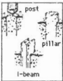
Figure 9. You can minimize damage to trees near foundations by using posts, pillars, or I-beams rather than foundation walls.
