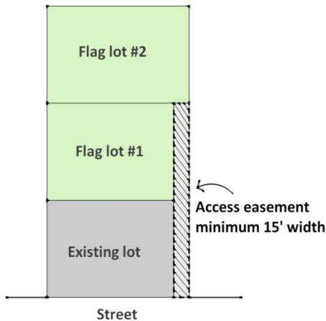
Figure 3: Multiple flag lots shall have a shared access easement
