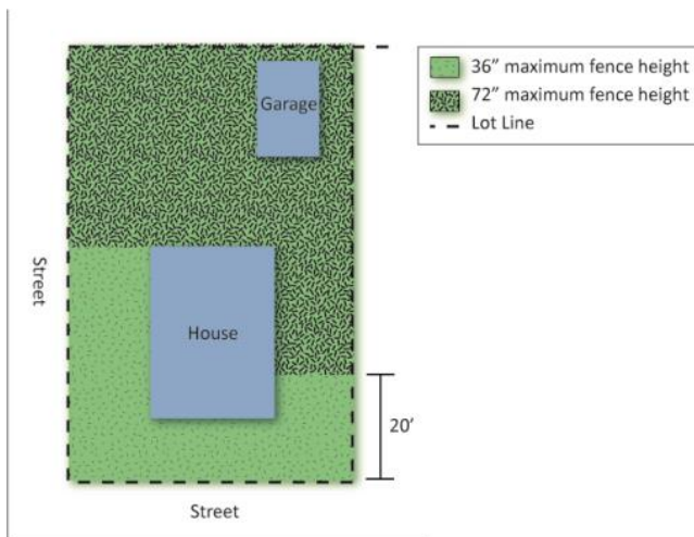
Figure 2: Example of Exempt Corner Lot Fence Locations
