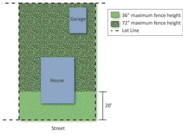
Figure 1: Example of Exempt Interior Lot Fence Locations
