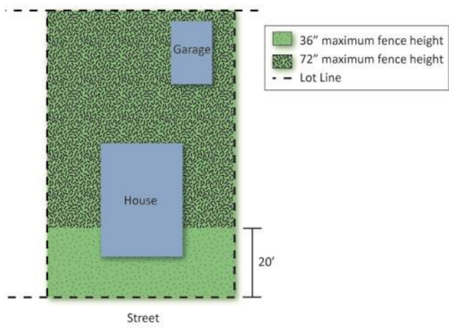
Figure 1: Example of Exempt Interior Lot Fence Locations
