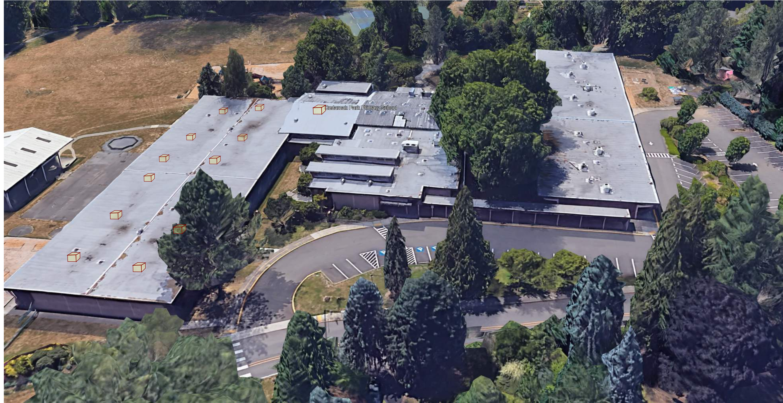
New south classroom RTU's to be similar to existing RTU layout on the north wing. Unit size: 80" L X 44 1/4" W X 50" H
