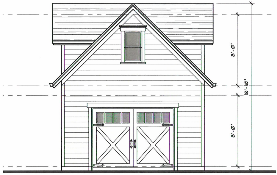
PROPOSED GARAGE ELEVATION ( SOUTH SIDE FACING ALLEY )
