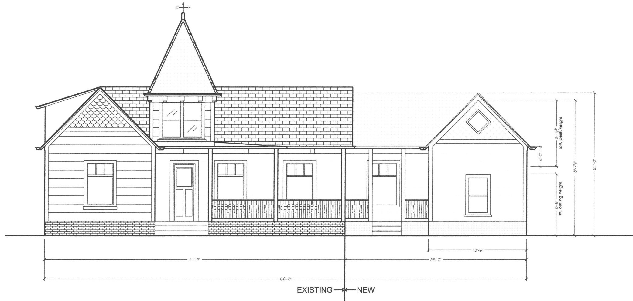
1 FRONT ELEVATION - PROPOSED NEW SCALE: 1/8" = 1'-0"
