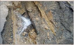
West Linn currently has 11.25 miles of asbestos-coated, or AC, pipe. When AC pipes break, the entire line must be replaced. The goal is to remove all AC pipe from the West Linn system.
