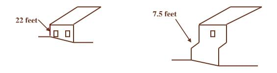
Sidewalls less than 22 feet high to eaves from average grade are exempt from popout/indentation requirement. Sidewall can resume vertically if set back 7.5 feet.
