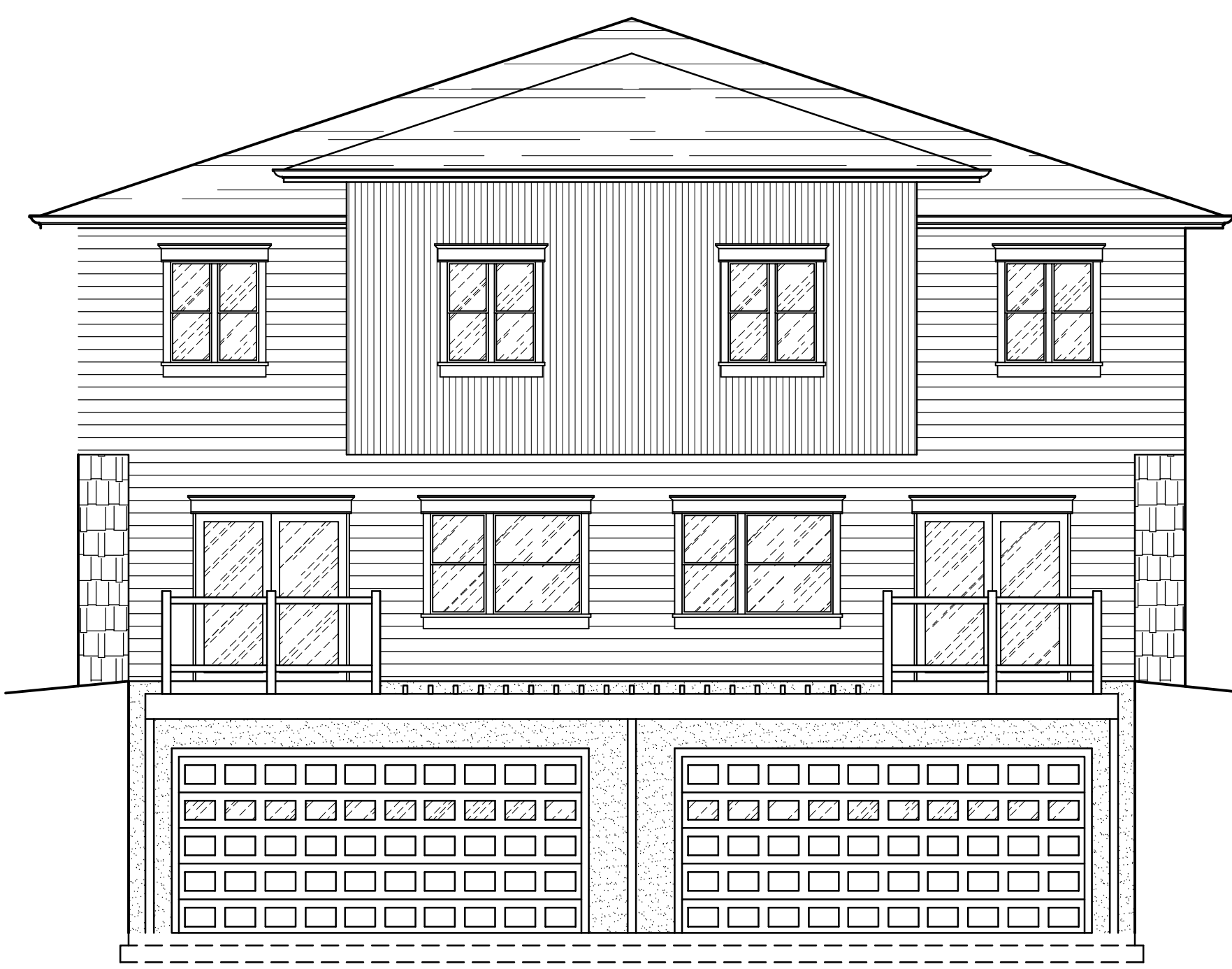
4 TYP. UNIT 'B' - REAR ELEVATION DRB2 3/16" = 1'-0"
