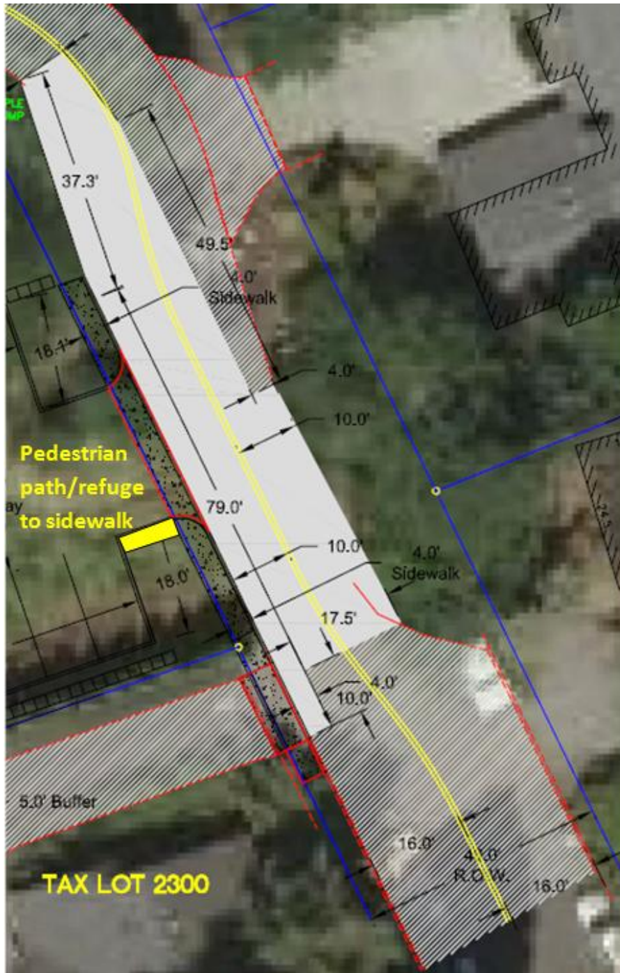
Figure 31: Hood Street proposed improvements
