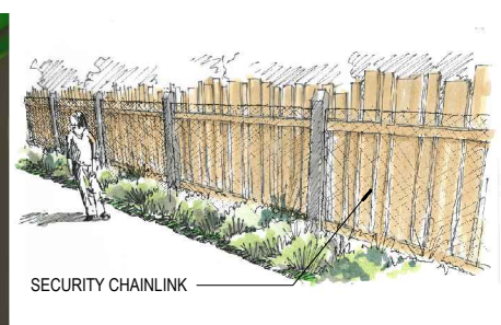
GOOD NEIGHBOR FENCE - VIEW FROM OWNER'S SIDE (SEE DETAIL 2, THIS SHEET)
