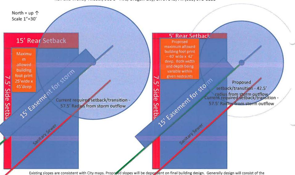
Existing slopes are consistent with City maps. Proposed slopes will be dependent on final building design. Generally design will consist of the driveway being located along the western boundary, and building to have a daylight basement allowing existing grades to remain.
