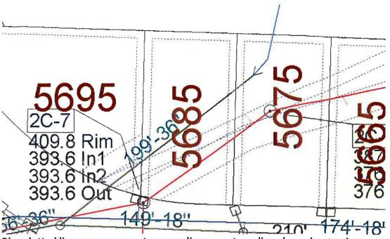
Blue dotted lines are easements, green lines are storm lines (opening to above ground section of creek next door), darker blue solid line is water line, red lines are sanitary sewer lines
