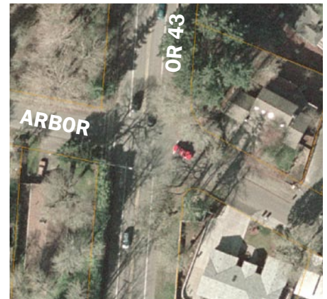
The OR 43/Arbor intersection is currently experiencing difficulties; existing ROW may allow for left turn lanes onto Arbor, but volumes do not warrant a signal to help traffic turning onto OR 43
