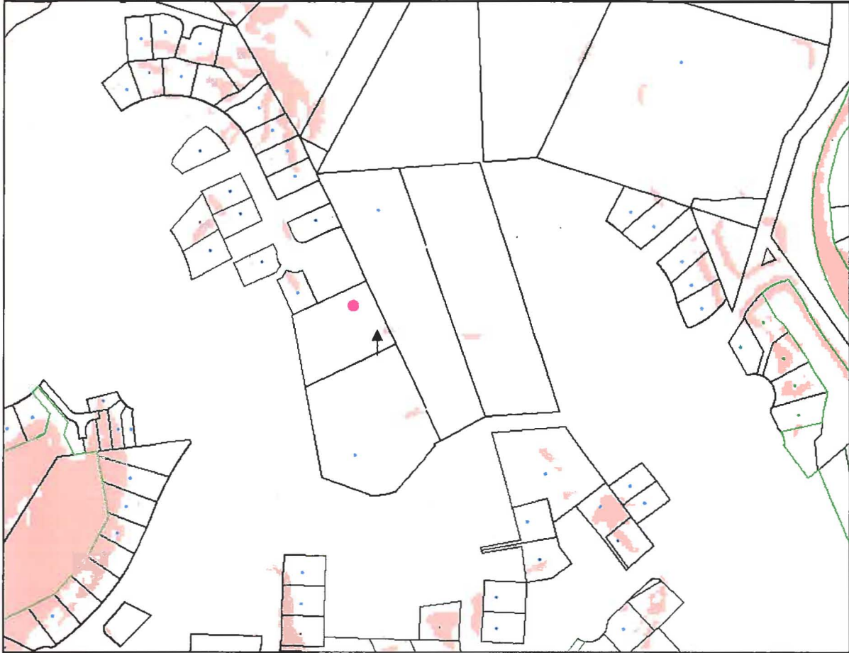
Excerpt of Map 17, Landslide Vulnerability Analysis, Page 52, West Linn Natural Hazards Mitigation Plan. Light pink represents landslide vulnerability areas. The darker pink dot identifies the site. The arrow points to where the northeast corner of the proposed structure will be located. The very small landslide area overlapping the site boundary starts approximately 8 feet east of where the structure is proposed.
