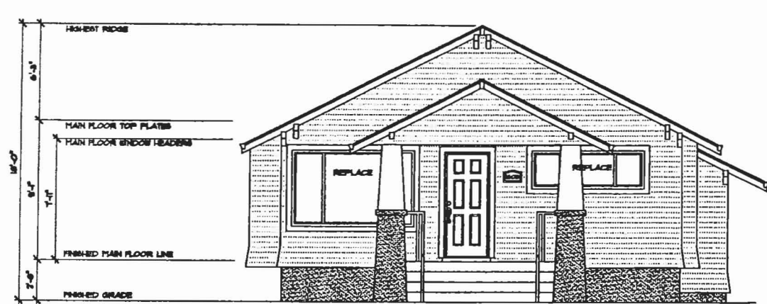
1 FRONT BUILDING ELEVATION A1.1 SCALE: 1/4" = 1'-0"
