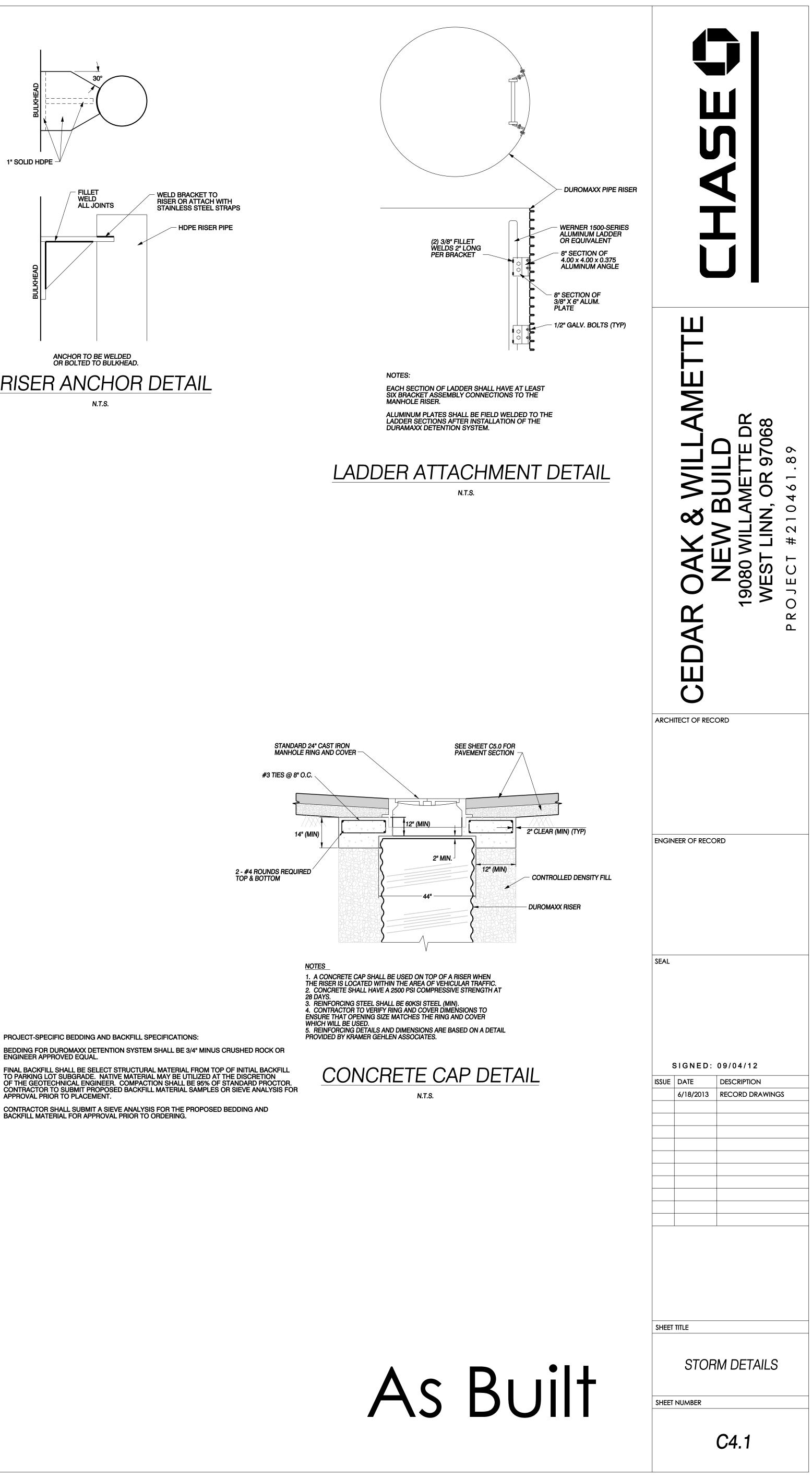
FINAL BACKFILL SHALL BE SELECT STRUCTURAL MATERIAL FROM TOP OF INITIAL BACKFILL TO PARKING LOT SUBGRADE. NATIVE MATERIAL MAY BE UTILIZED AT THE DISCRETION OF THE GEOTECHNICAL ENGINEER. COMPACTION SHALL BE 95% OF STANDARD PROCTOR. CONTRACTOR TO SUBMIT PROPOSED BACKFILL MATERIAL SAMPLES OR SIEVE ANALYSIS FOR APPROVAL PRIOR TO PLACEMENT. CONTRACTOR SHALL SUBMIT A SIEVE ANALYSIS FOR THE PROPOSED BEDDING AND BACKFILL MATERIAL FOR APPROVAL PRIOR TO ORDERING.
